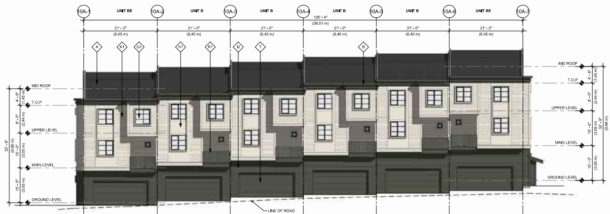
1 BUILDING 10A - WEST ELEVATION 1:100
