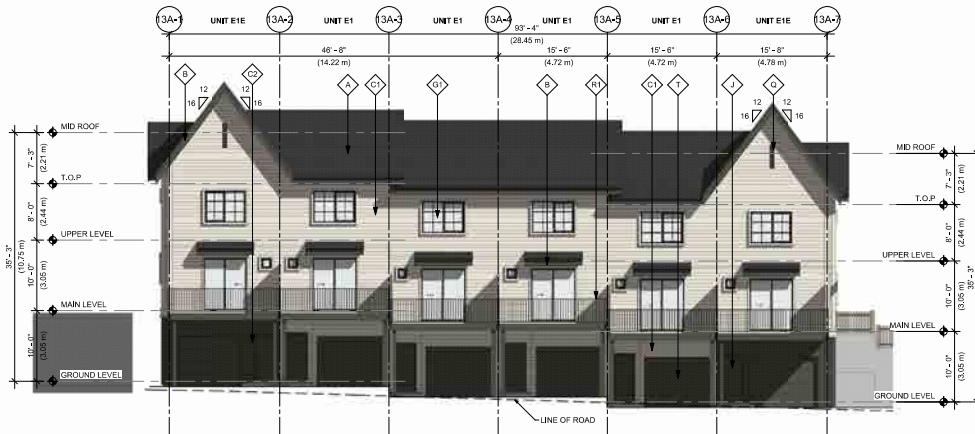
1 BUILDING 13A - NORTH ELEVATION 1:100
