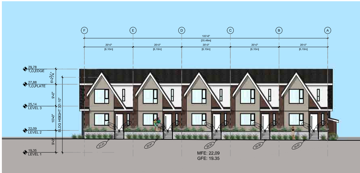
3 BUILDING 1- WEST ELEVATION SCALE: 1/16" = 1'-0"
