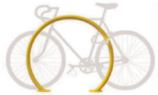
D2 BIKE RACK N.T.S. MANUFACTURER: DENO MODEL: ROUND COLOUR: ORANGE/BLUE QUANTITY: 5 OR APPROVED EQUAL
