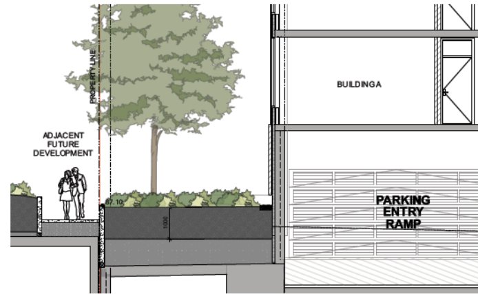
5 SECTION THROUGH PLANTER WEST OF BUILDING A AND ADJACENT SITE (LOOKING NORTH) 1:50
