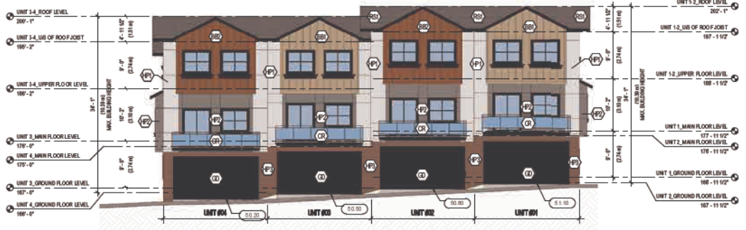
1 BUILDING-1 NORTH ELEVATION SCALE: 1/8"=1'-0"
