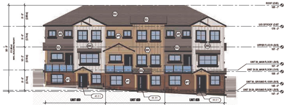
2 BUILDING-08 EAST ELEVATION SCALE: 1/8" = 1'-0"
