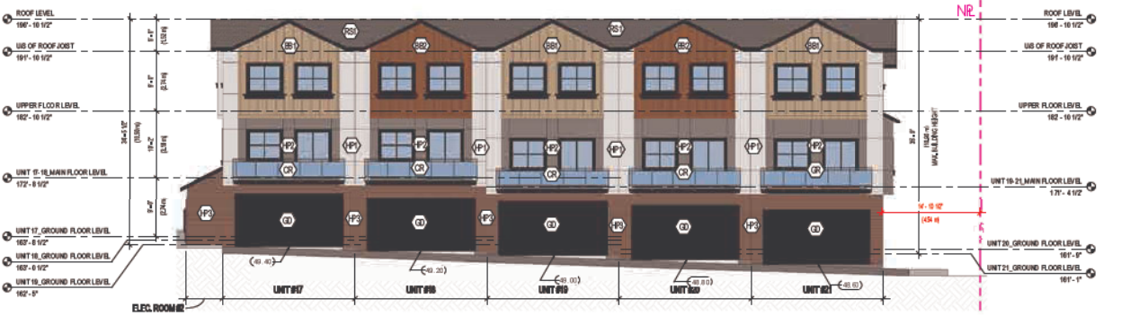
2 BUILDING-5 EAST ELEVATION SCALE: 1/8" = 1'-0"
