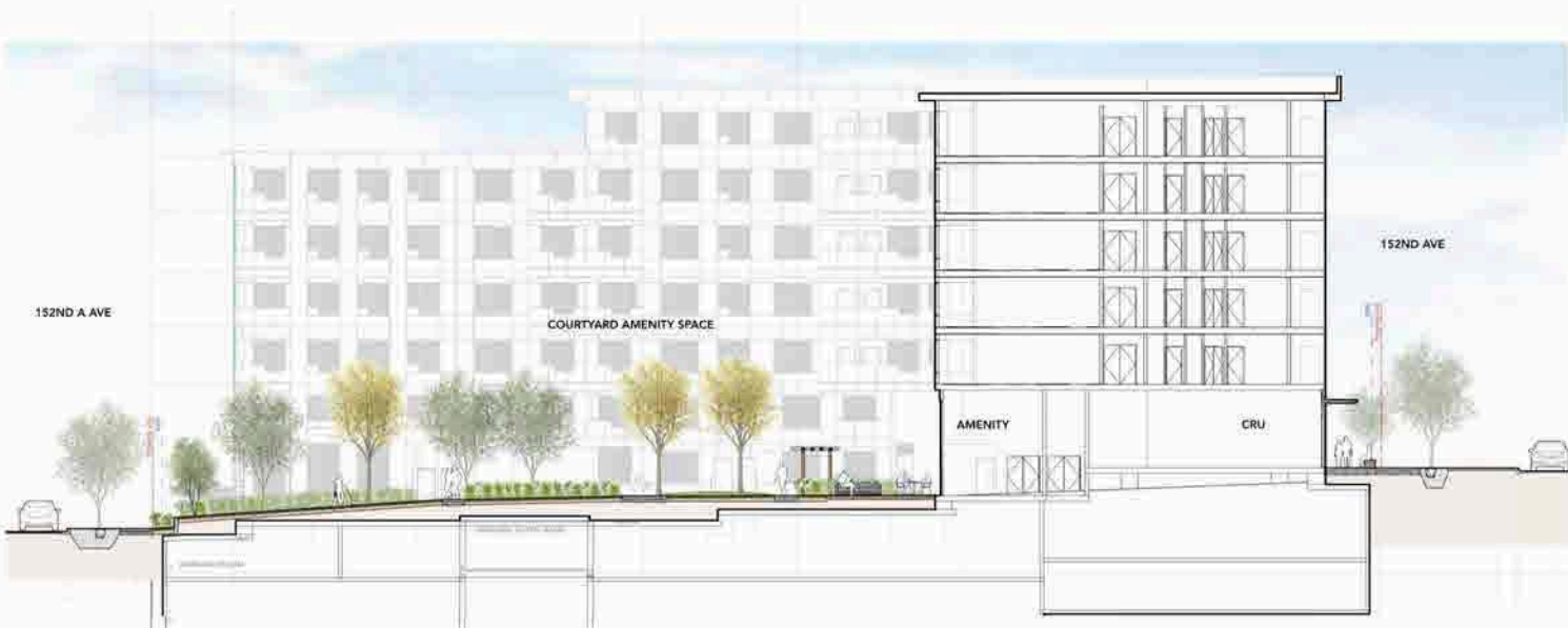
2 Section Through Courtyard Looking South Scale: 1/100
