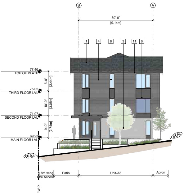
2 SOUTH ELEVATION (19 Avenue) BUILDING-1
