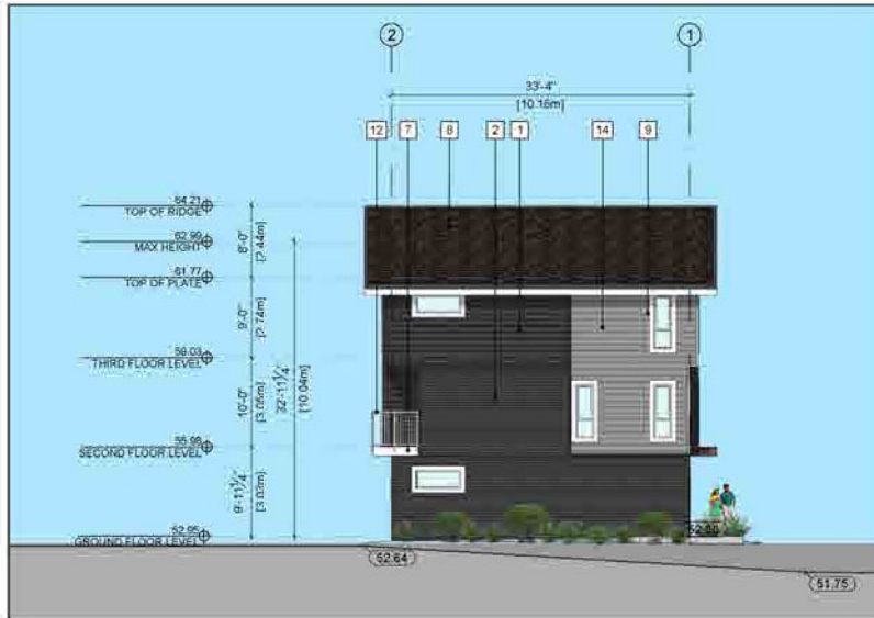
2 BUILDING 7 EAST ELEVATION
