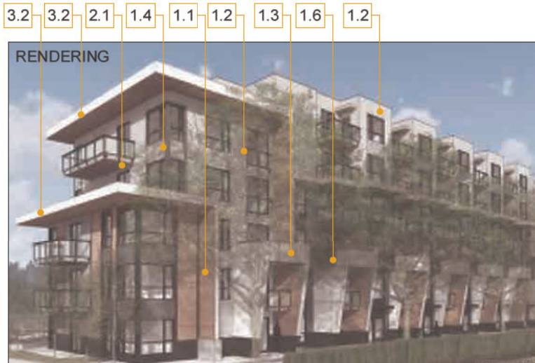
1.3 Fibre Cement Panel w/ Reveal - Arctic White
