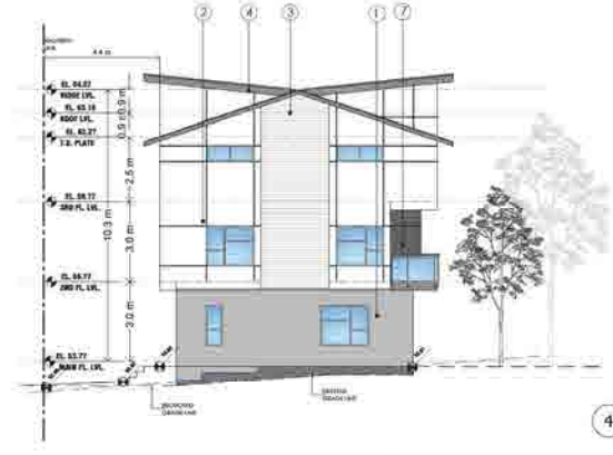
2 NORTH (FACING 25 AVE.) ELEVATION Scale: 1/8"=1'-0"
