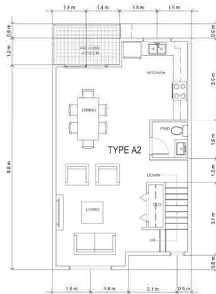
TYPE A2 2nd FLOOR AREA = 561.39 SQ FT = 51.90 SQ M
