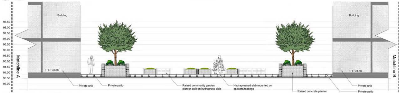
2 CROSS-COURT SECTION - COURTYARD Scale 1:100
