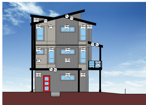
3 COLORED EAST ELEVATION (164 STREET) DP-A-6.17 1/8" = 1'-0"
