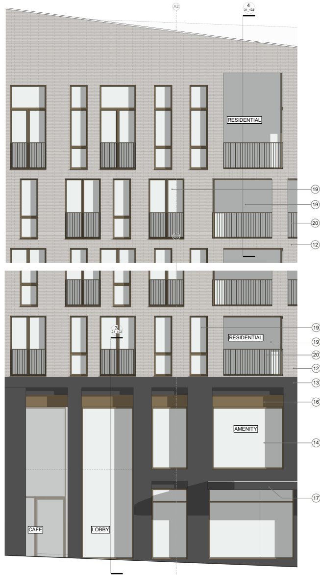
① Elevation Block A Lower 1:50
