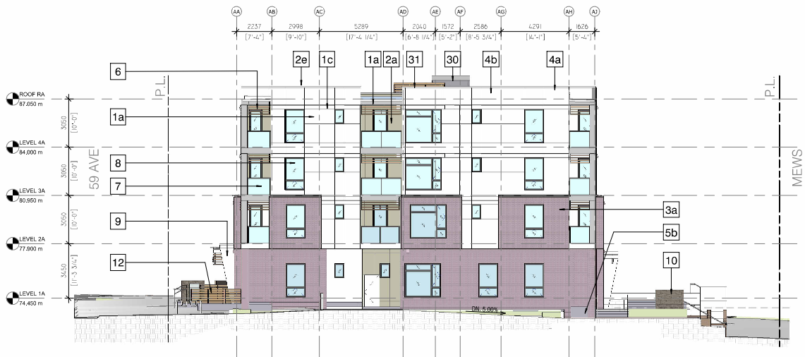
E EAST ELEVATION BUILDING A SCALE: 1 : 100
