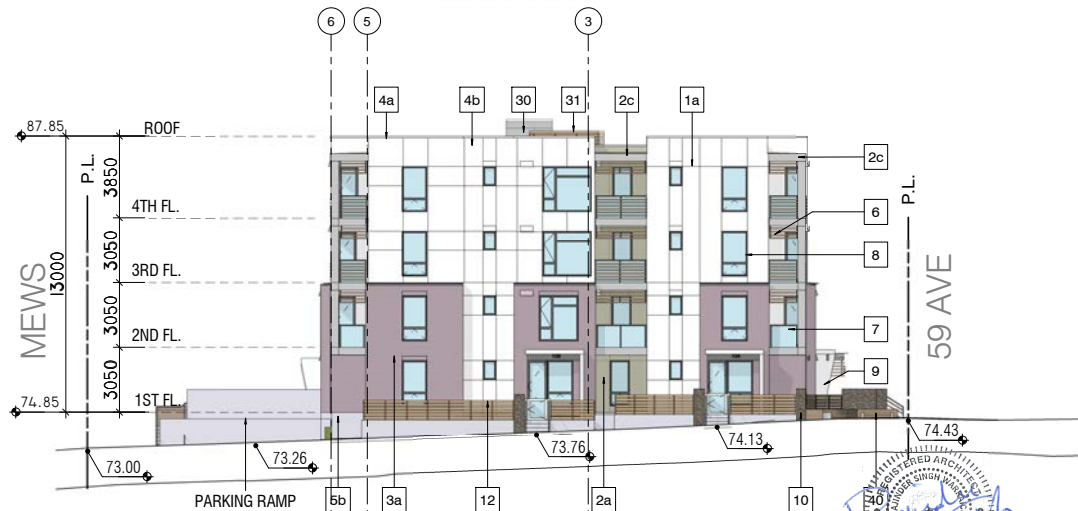
2 BUILDING A WEST ELEVATION (143 ST) SCALE: 1:96
