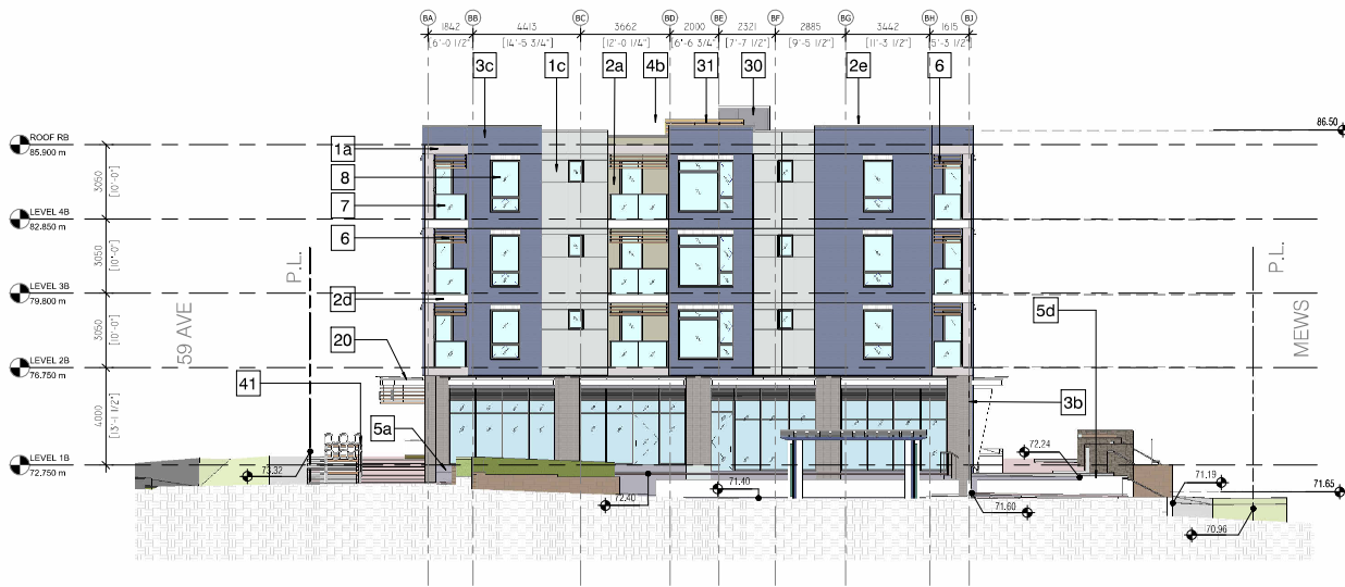
1 EAST ELEVATION BUILDING B SCALE: 1 : 100
