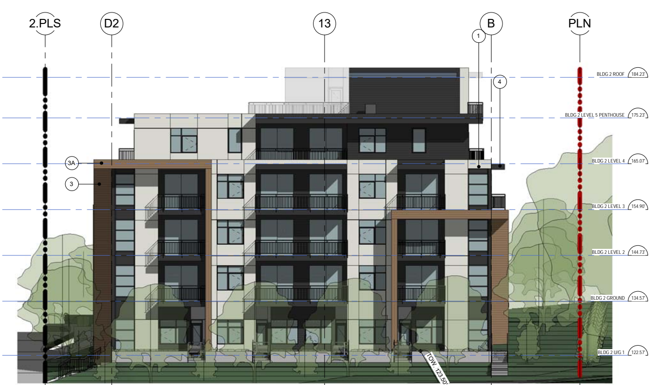
① BUILDING 2/BLOCK B (EAST) EAST ELEVATION 1" = 10'-0"
