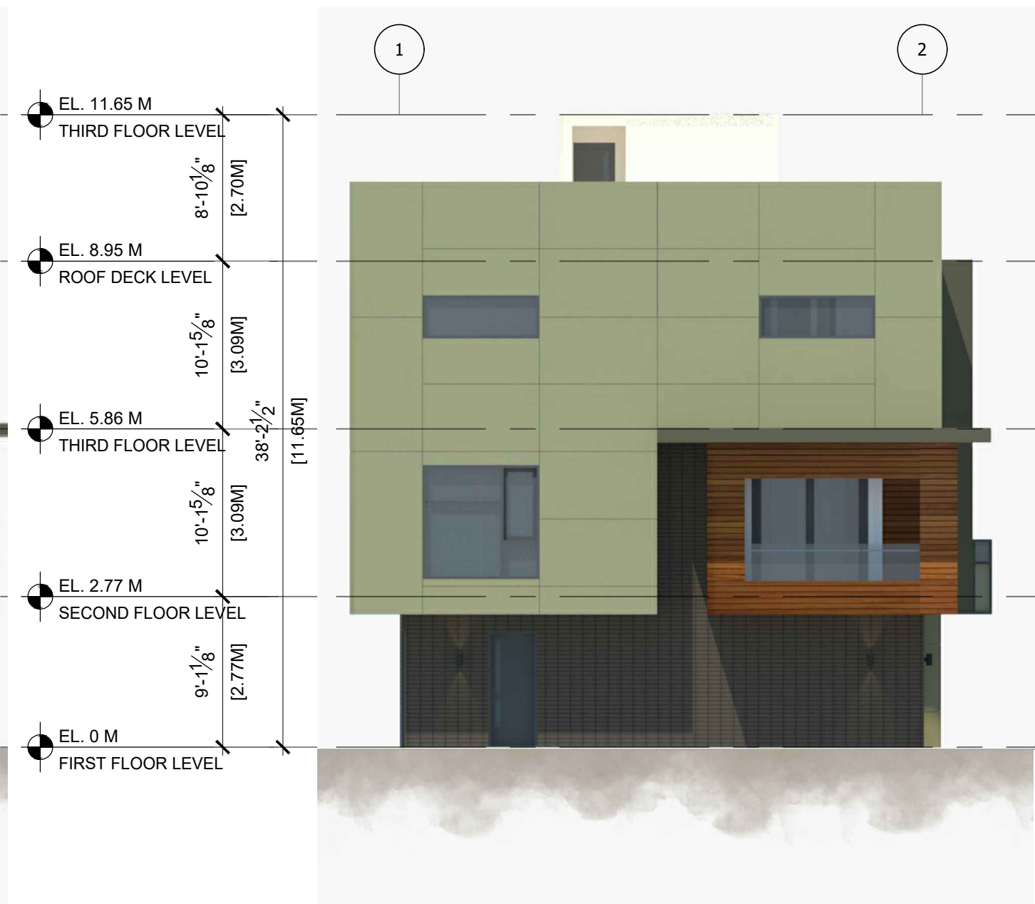
2 BUILDING 5 - WEST ELEVATION SCALE 1/8" = 1'-0"
