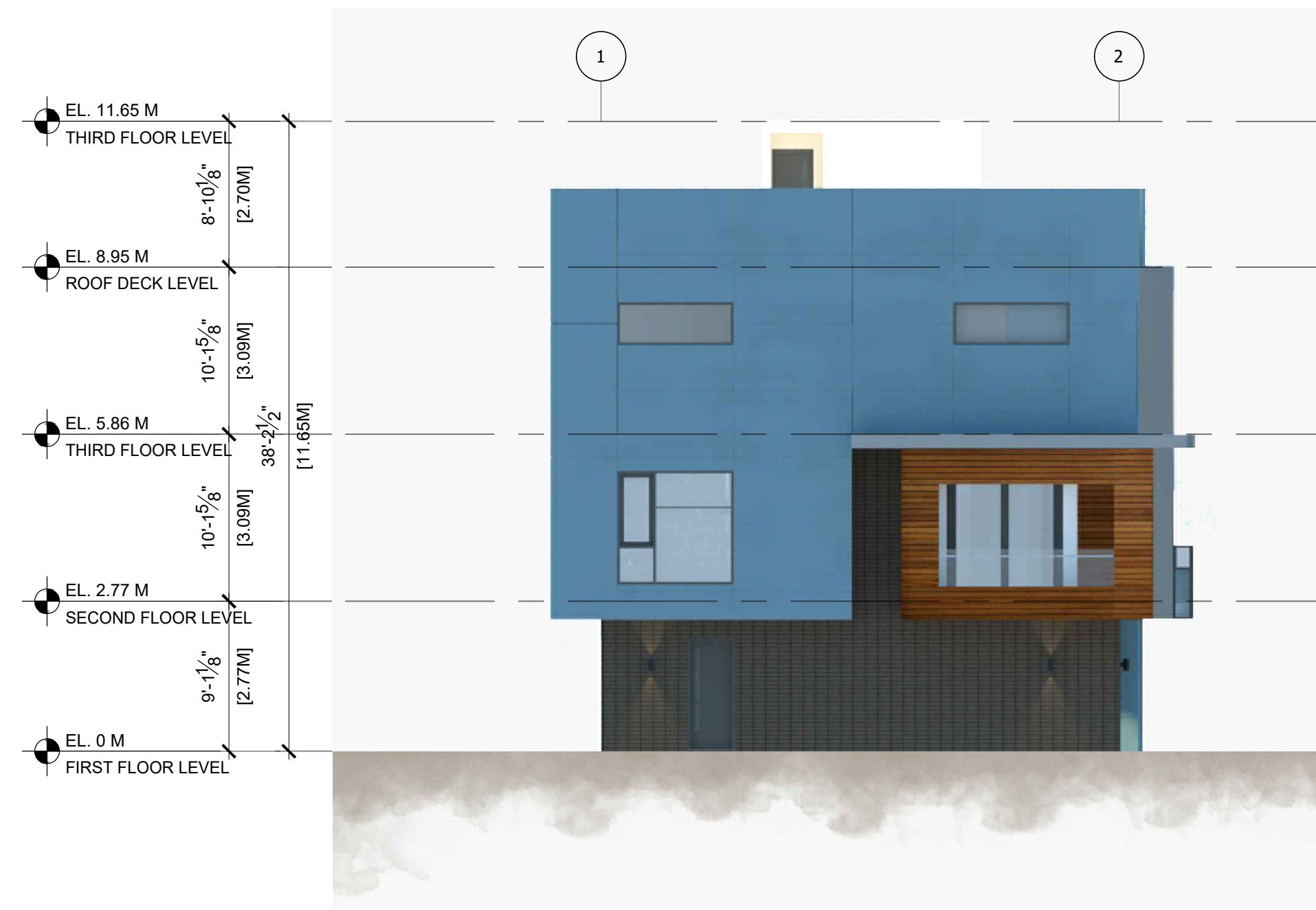
2 BUILDING 1 - EAST ELEVATION SCALE 1/8" = 1'-0"
