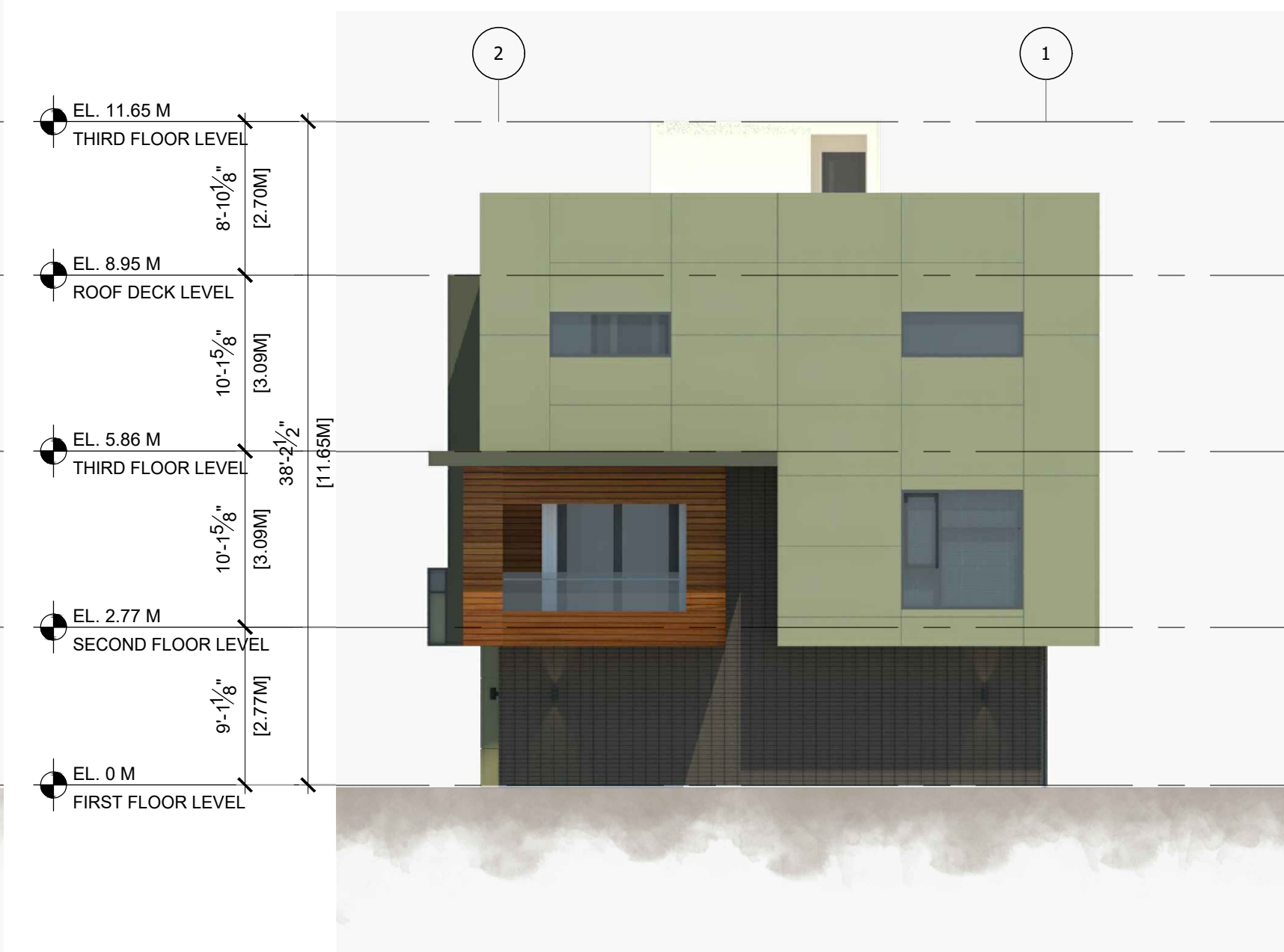
4 BUILDING 3 - WEST ELEVATION SCALE 1/8" = 1'-0"
