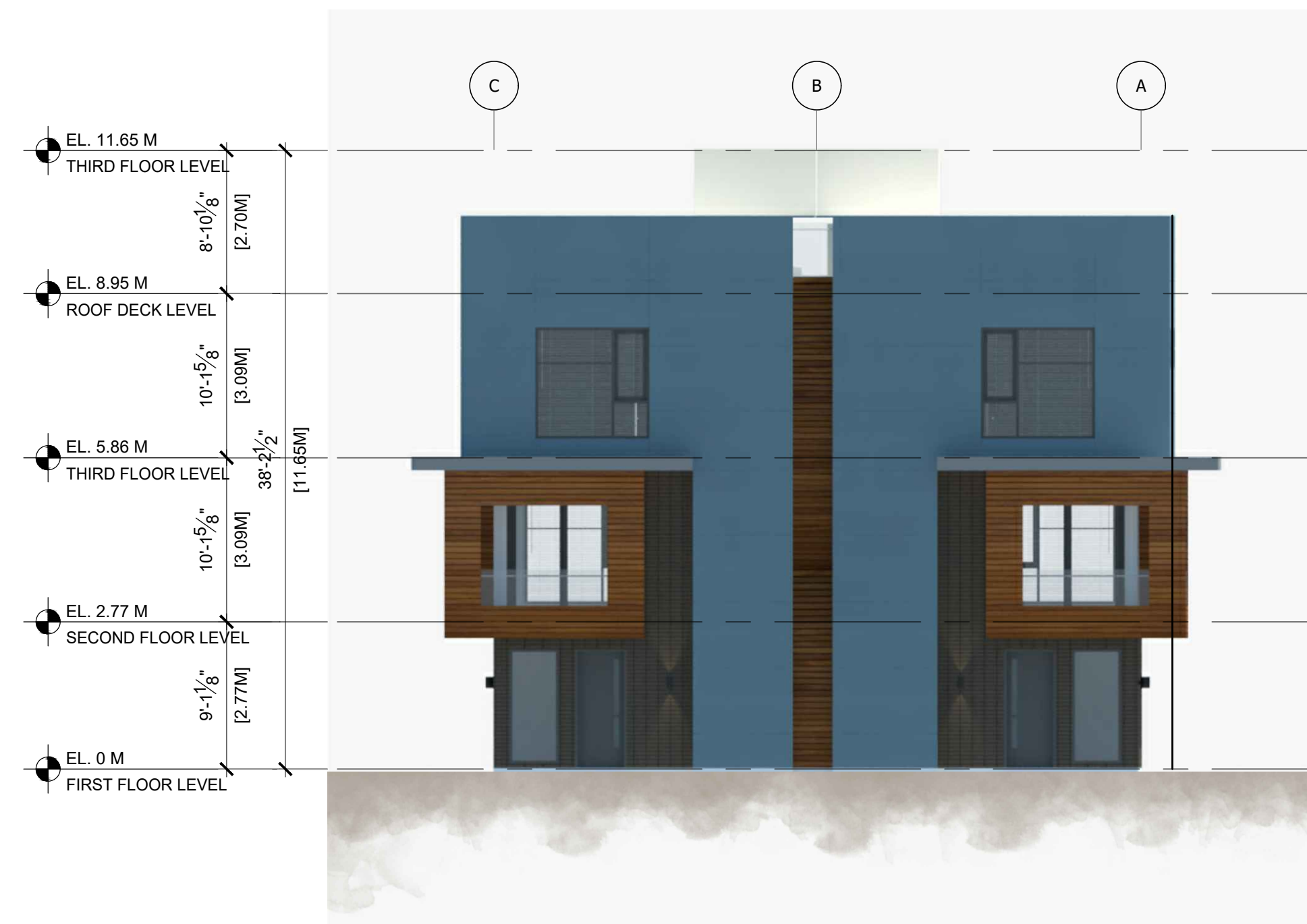
1 BUILDING 1 - NORTH ELEVATION SCALE 1/8" = 1'-0"
