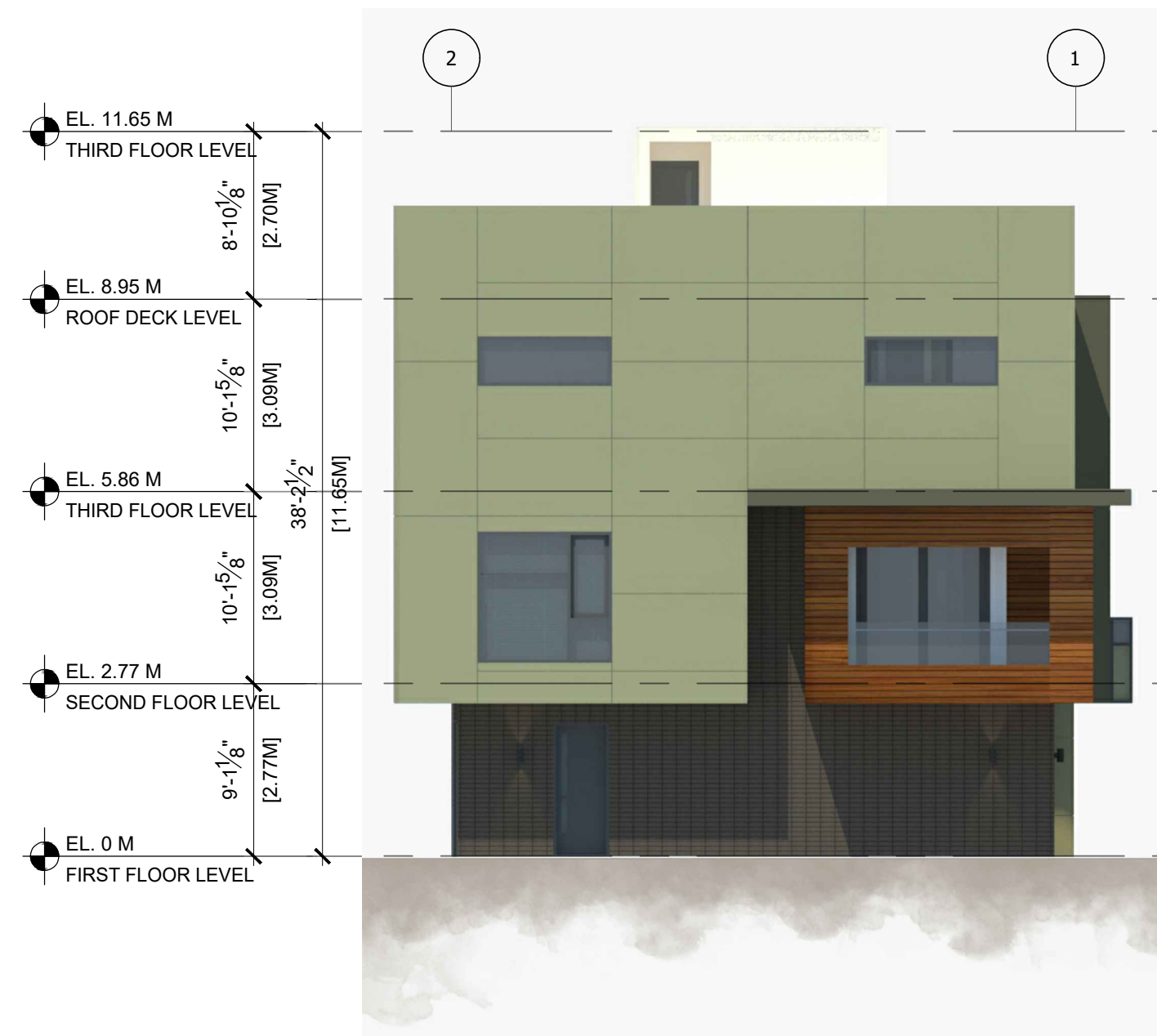
2 BUILDING 7 & 8 - NORTH ELEVATION SCALE 1/8" = 1'-0"
