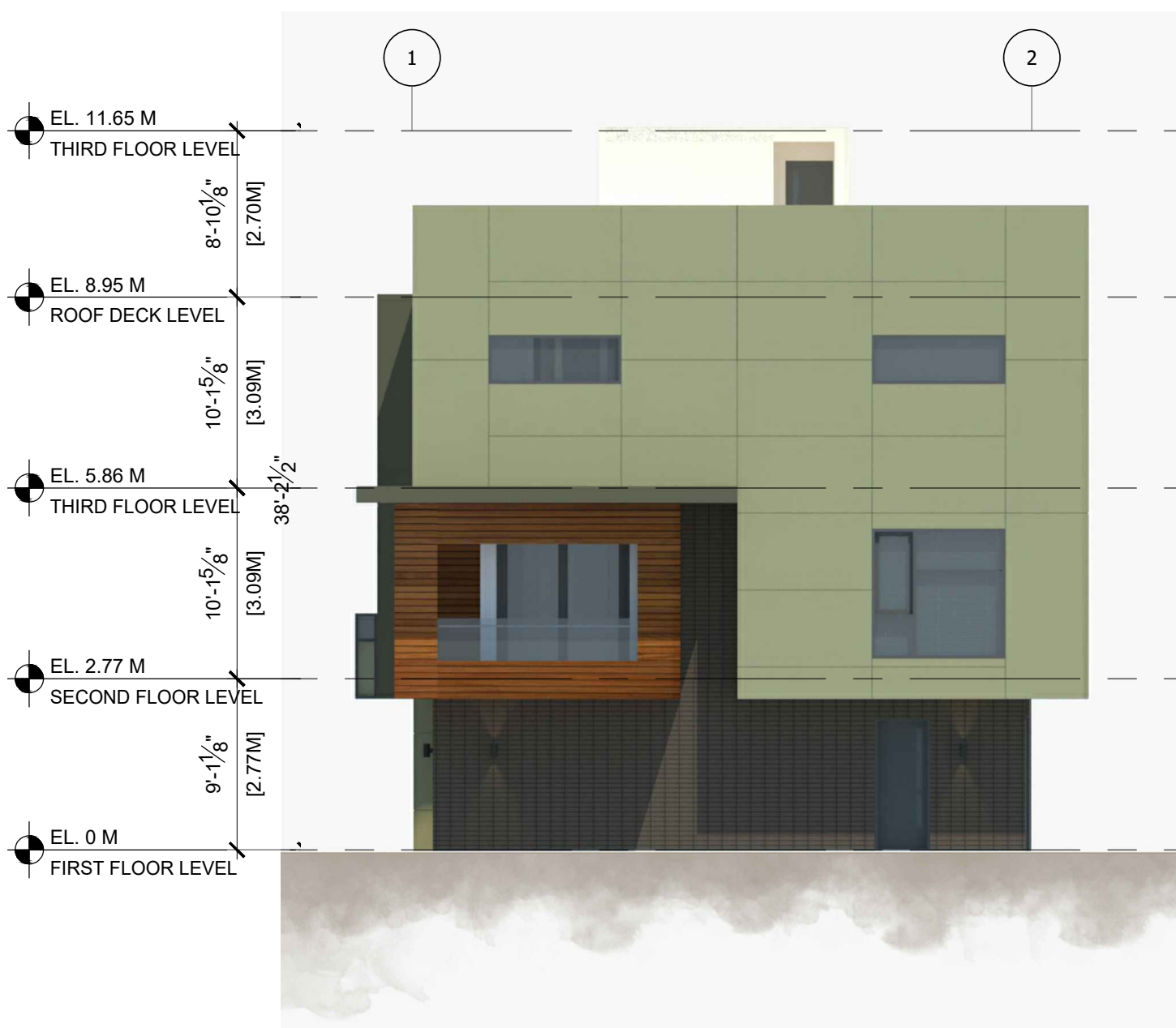
4 BUILDING 7 & 8 - SOUTH ELEVATION SCALE 1/8" = 1'-0"
