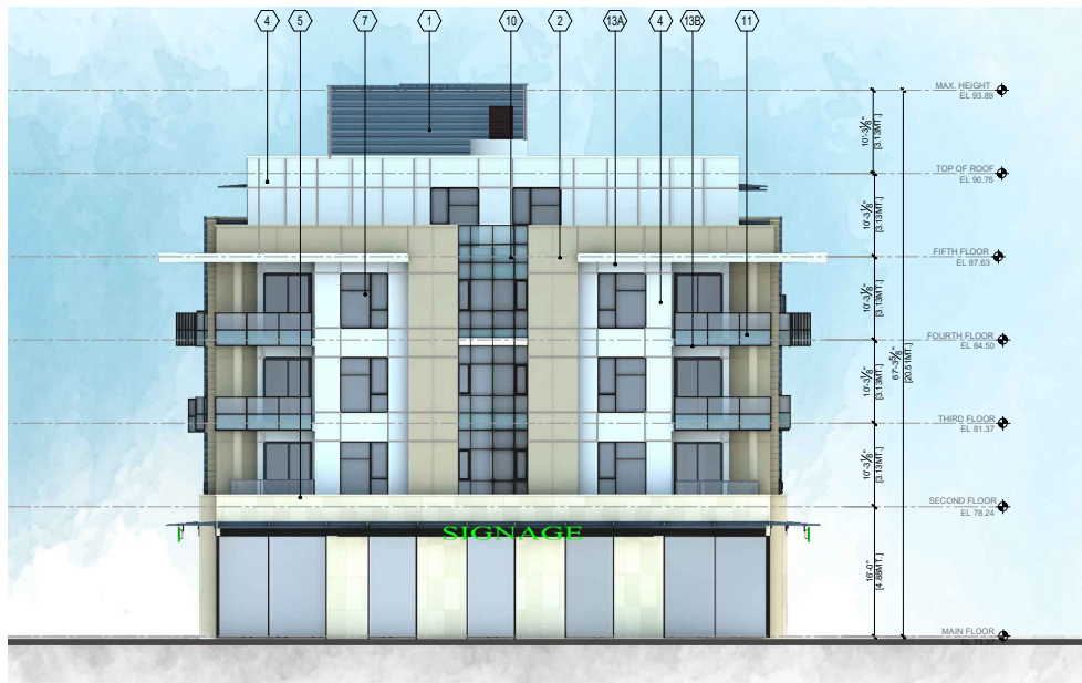
1 SOUTH SIDE ELEVATION(BUILDING#1) N.T.S.
