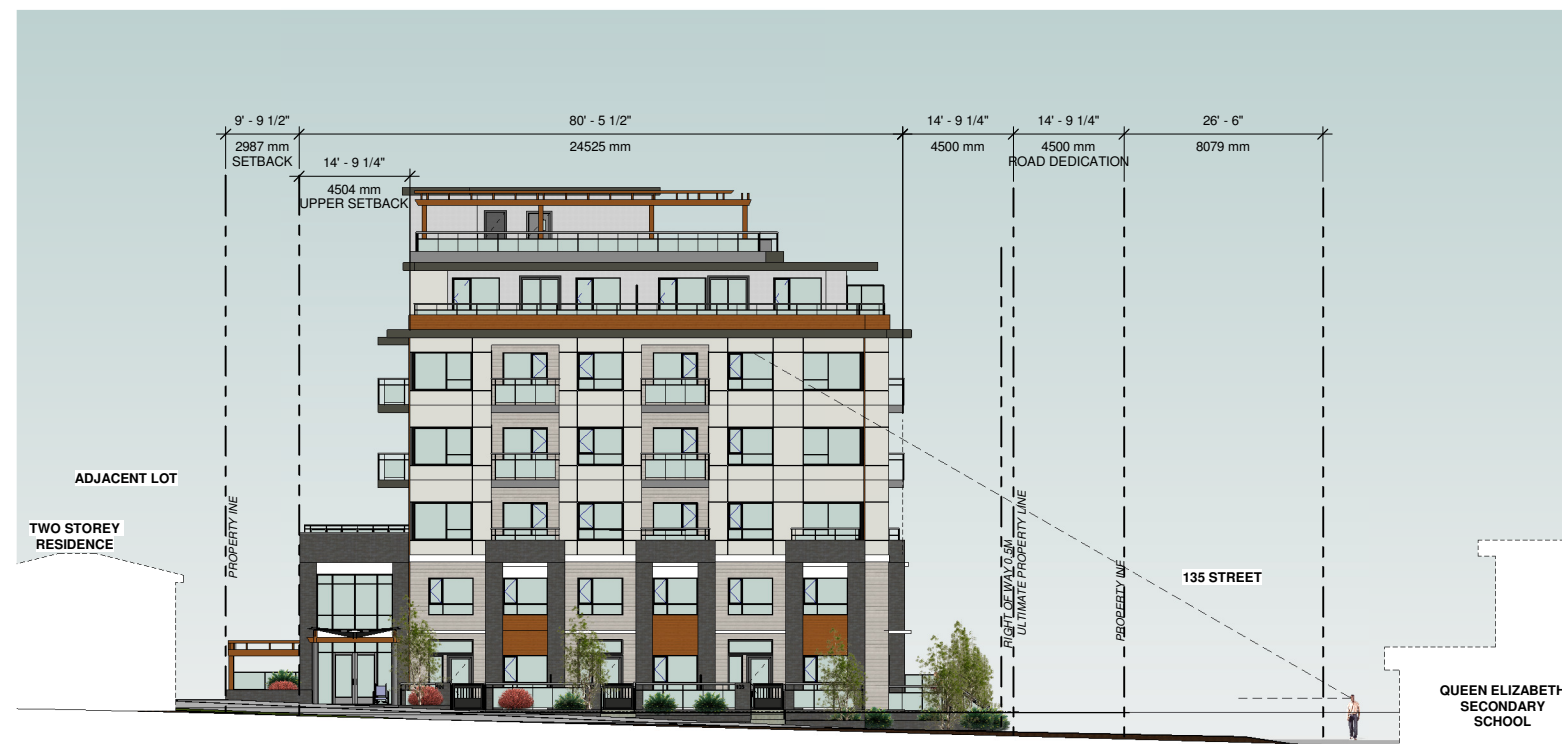
SOUTH ELEVATION (STREETSCAPE ALONG 94a AVENUE) 2 3/32" = 1'-0"
