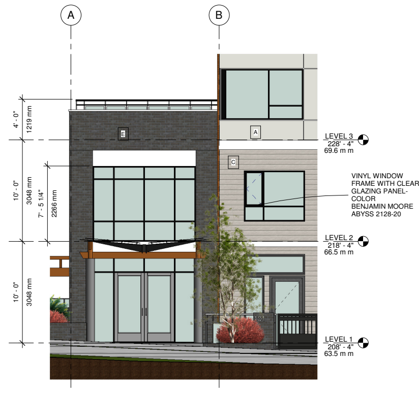
3 PARTIAL ELEVATION (MAIN ENTRANCE) 1/4" = 1'-0"
