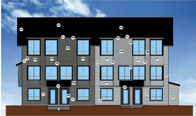
1 COLOURED SOUTH ELEVATION DP-5.32 / 1/8" = 1'-0"
