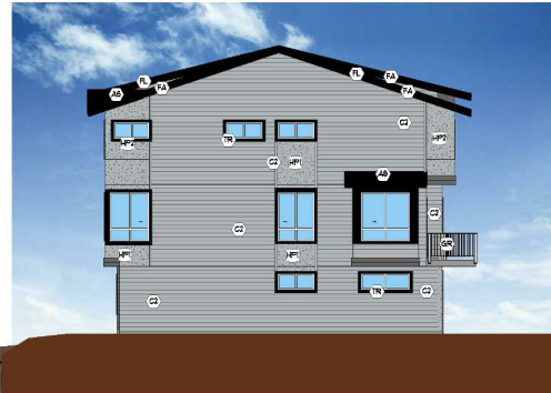
3 COLOURED EAST ELEVATION
