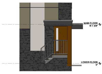
3 NORTH ELEVATION (ALDER PLACE) BLDG 1 & 4 SCALE: 1/4" = 1'-0" BUILDING 1: UNIT 01 ONLY BUILDING 4: UNIT 18 ONLY
