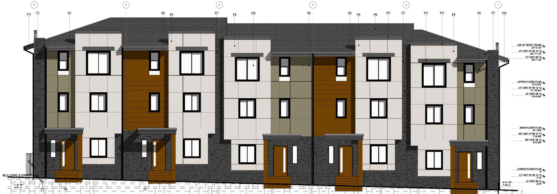
SOUTH ELEVATION- BLDG 5 SCALE: 1/4" = 1'-0"
