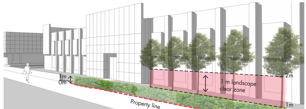
Providing one meter landscape clear zone between top of ground plantings and bottom of tree canopy for visibility.
