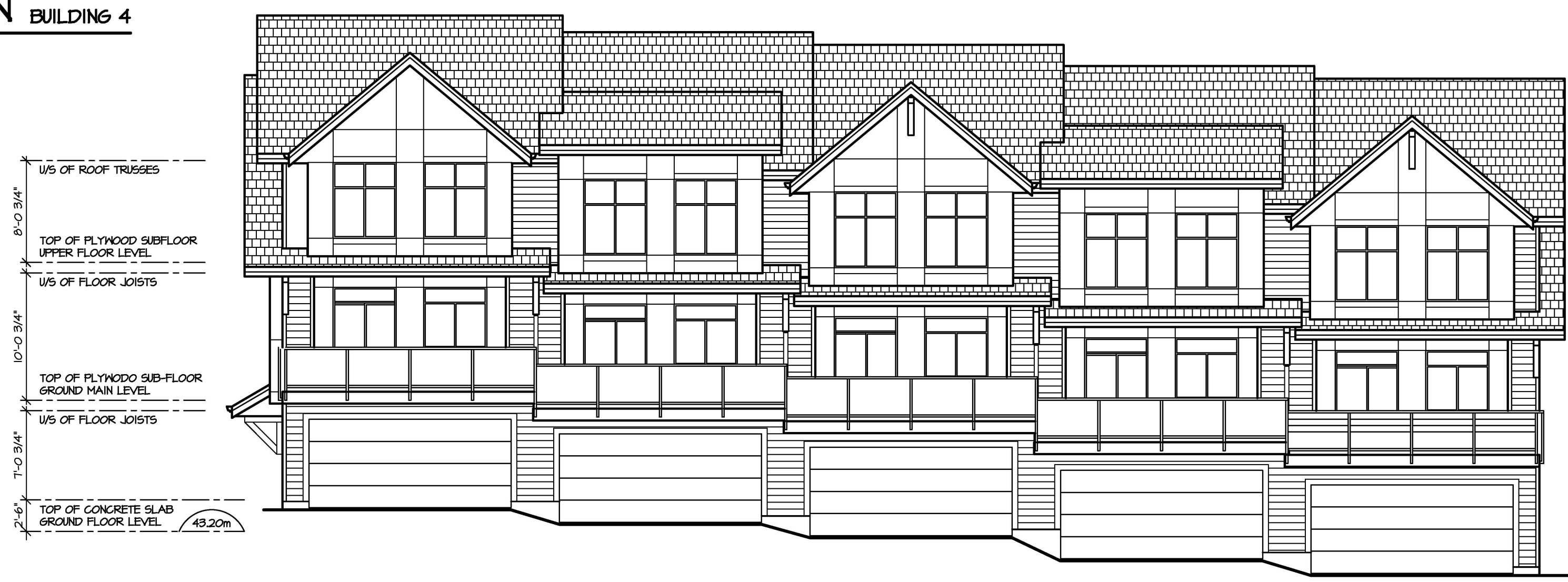
EAST ELEVATION BUILDING 4 SCALE: 1/8" = 1'-0"
