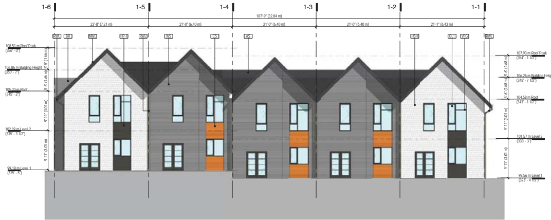
② Building 1 - East Elevation 1/8" = 1'-0"
