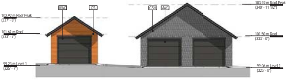
③ Garage - North Elevation 1/8" = 1'-0"
