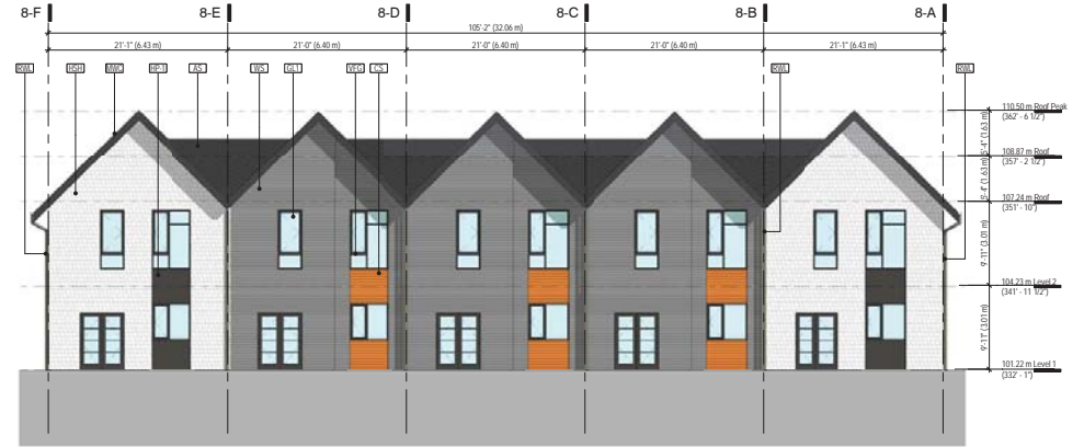
① Building 8 - North Elevation 1/8" = 1'-0"
