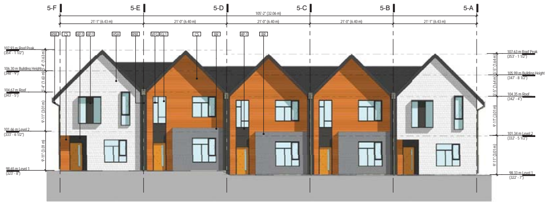
① Building 5 - North Elevation 1/8" = 1'-0"
