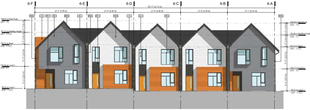
① Building 6 - North Elevation 1/8" = 1'-0"
