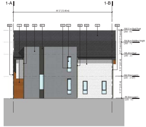
③ Building 1 - South Elevation 1/8" = 1'-0"
