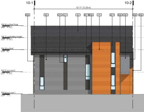
④ Building 10 - West Elevation 1/8" = 1'-0"
