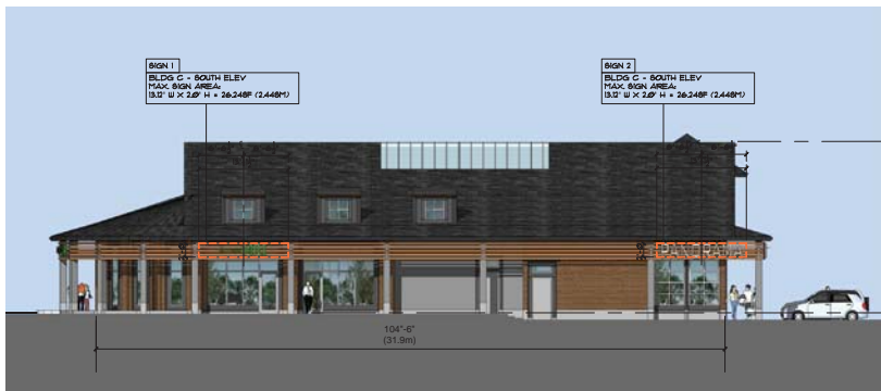
4 SOUTH ELEVATION CSA SCALE: 1/8" = 1'-0"
