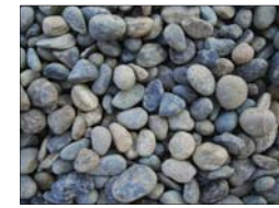
AGGREGATE #3 RIVER ROCK SIZE: 40-50MM \phi
