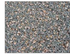
AGGREGATE #2 BLUE METAL AGGREGATE SIZE: 10-20MM \phi
