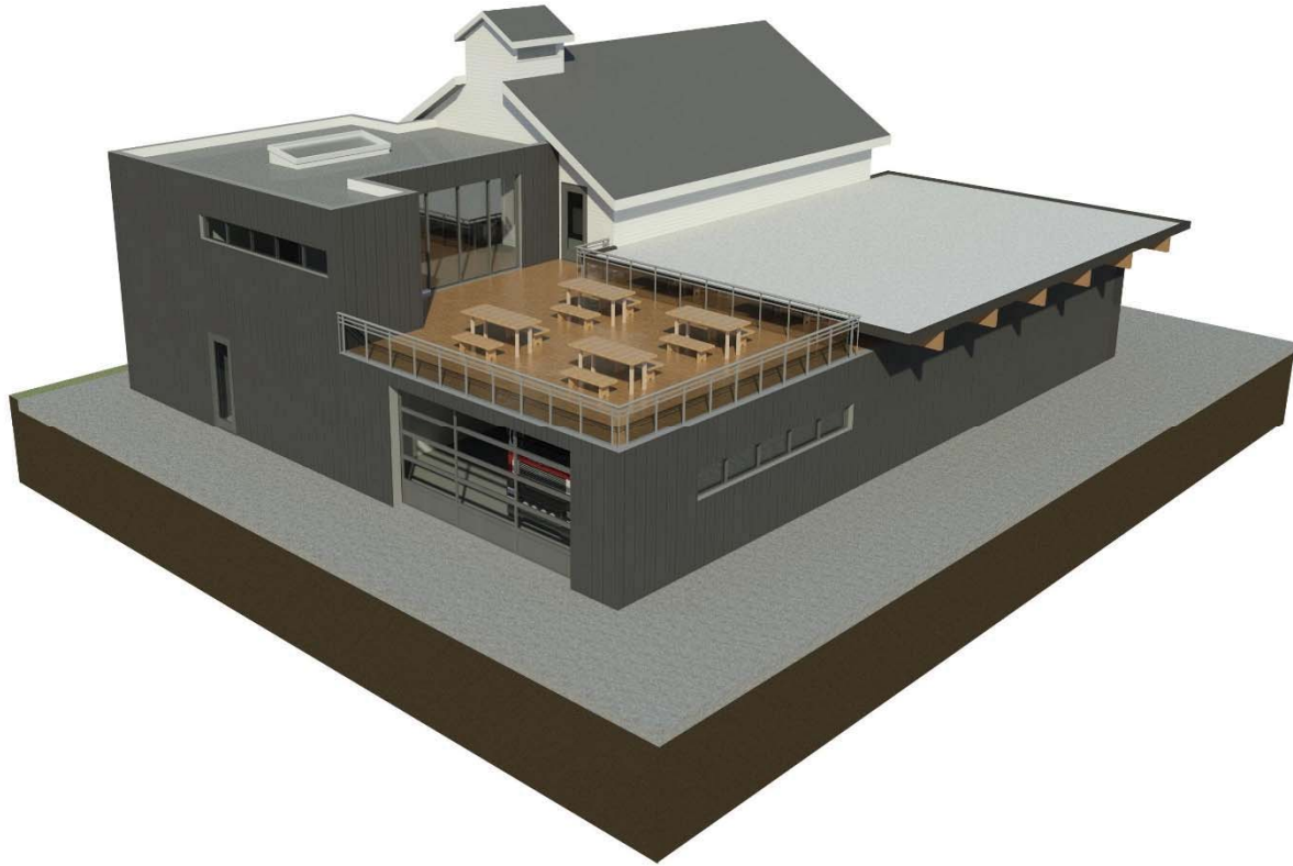
above: 3D model of the proposed rehabilitation from the Northwest corner. The new addition steps in from the heritage building, and drops below the roofline. It is visibly discernable from the heritage building with its contemporary cladding and blocky massing.
