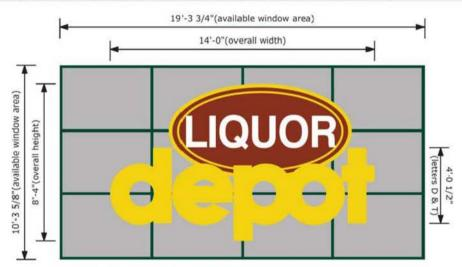
MANUFACTURE AND INSTALL...EXTERIOR ONE SET OF SELF-CONTAINED LED-ILLUMINATED CHANNEL LETTERS AND SHAPES INSTALLED ONTO EXISTING WINDOW MULLIONS ON THE PARKING LOT ELEVATION NOTE: OVAL AND LETTERS E, P, & O ARE TO BE BUILT AS ONE COMPLETE CHANNEL SHAPE. LETTERS "D & T" TO BE SEPARATE CHANNEL LETTERS.
