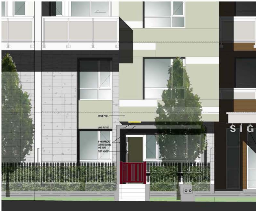
1 A4.3 DETAIL ELEVATION OF TOWNHOUSE SCALE 1/25
