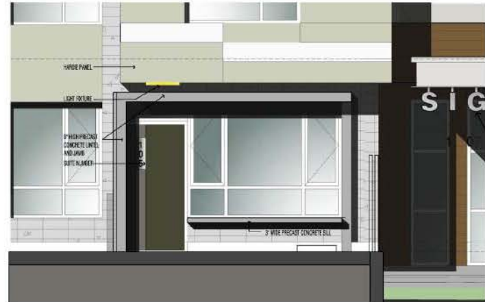
3 A4.3 DETAIL ELEVATION OF TOWNHOUSE ENTRY SCALE 1/25
