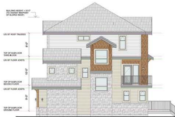
NORTH ELEVATION (SIDE)
