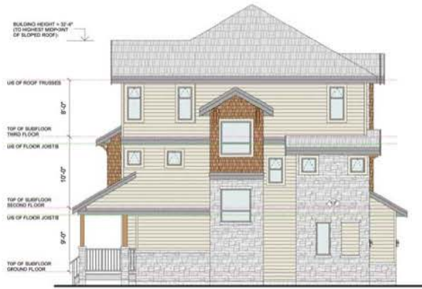
NORTH ELEVATION (SIDE)
