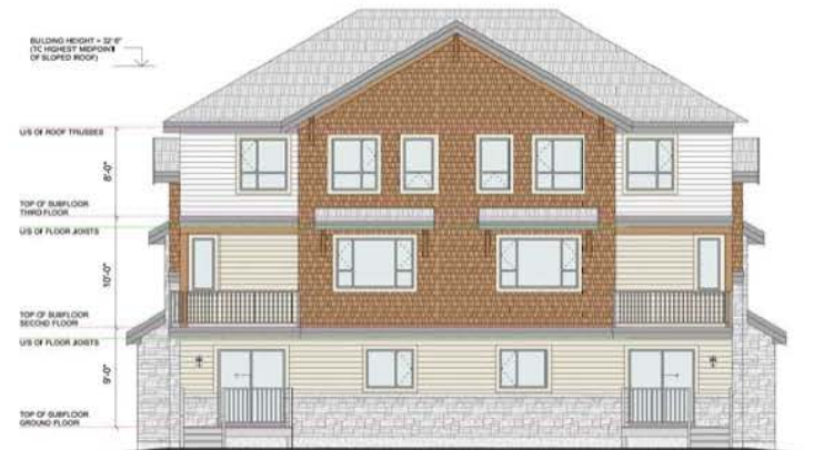
EAST ELEVATION (FACING 156TH STREET)
