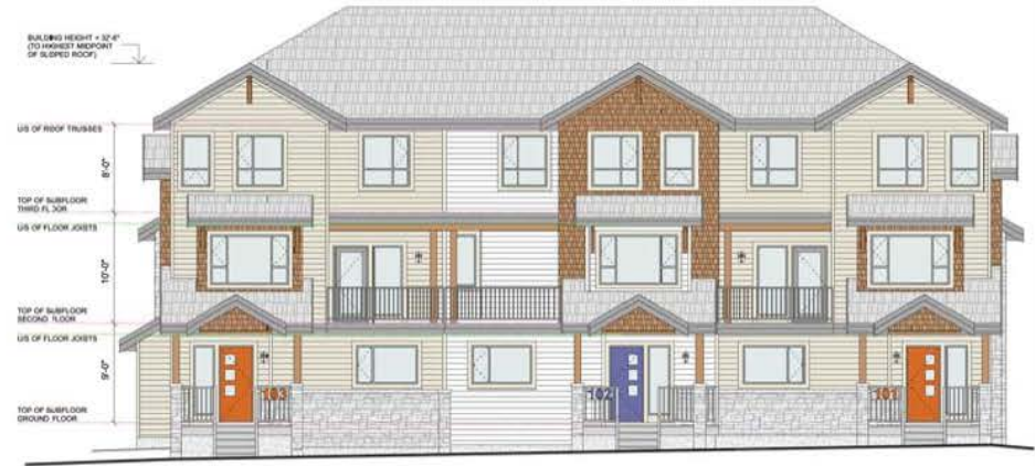
EAST ELEVATION [FACING KING GEORGE HIGHWAY]
