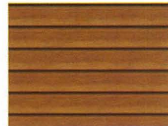
5 | CEDAR SIDING 1x6 T&G select bevelled edge cedar with water based stain - colour to match Sikkens BRD natural oak
