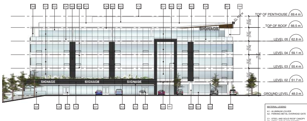
1 BUILDING B - NORTH ELEVATION A302 1/16" = 1'-0"
