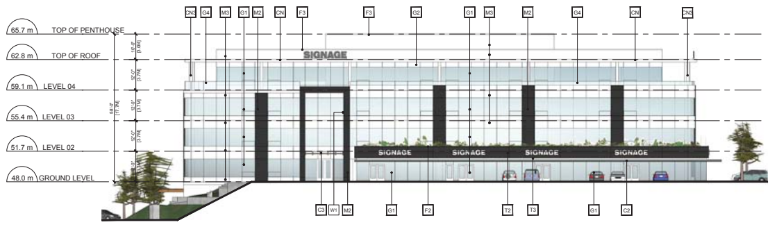
2 BUILDING A - EAST ELEVATION A301 1/32" = 1'-0"
