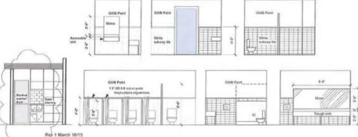
BATHROOM WALL ELEVATIONS Scale: 1/4" = 1'-0"
