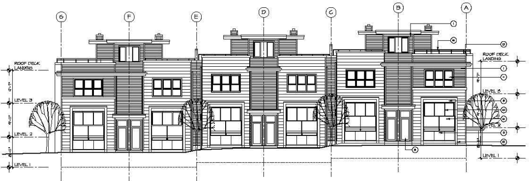
1 BUILDING TYPE 'D' - FRONT (EAST) ELEVATION SCALE: 1/8" = 1'-0"
