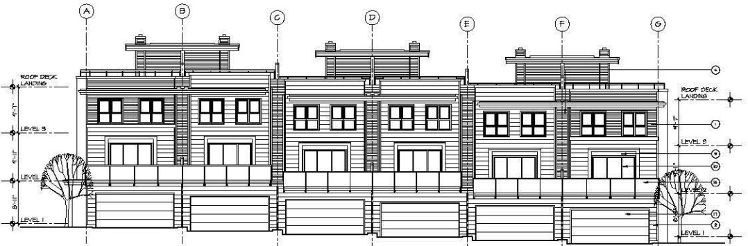
2 BUILDING TYPE 'D' - REAR (WEST) ELEVATION SCALE: 1/8" = 1'-0"
