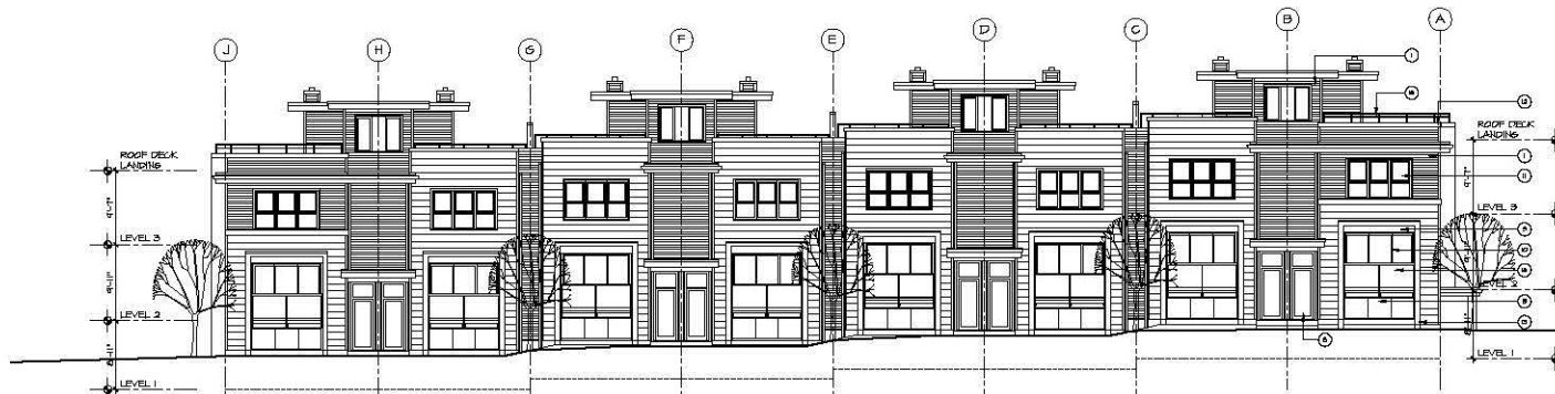
1 BUILDING TYPE '6' - FRONT (EAST) ELEVATION SCALE 1/8" = 1'-0"
