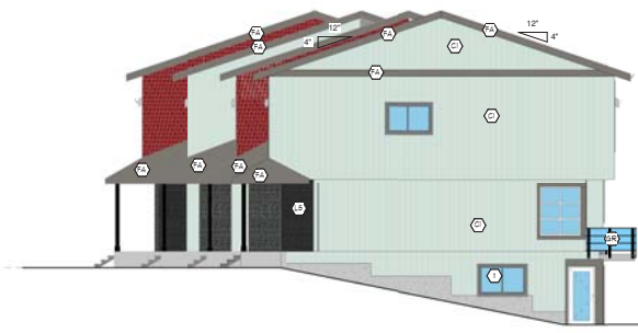
4 COLOURED WEST ELEVATION DP-1.12 1/8" = 1'-0"
