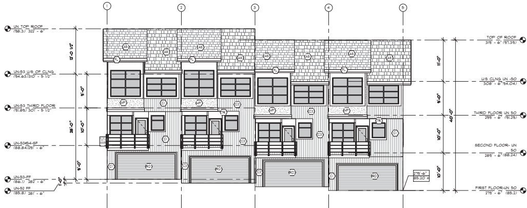
1 SOUTH ELEVATION DP-5.111 1/8" = 1'-0"
