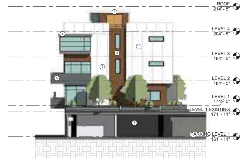
③ Building 6, East Elevation 3/32" = 1'-0"
