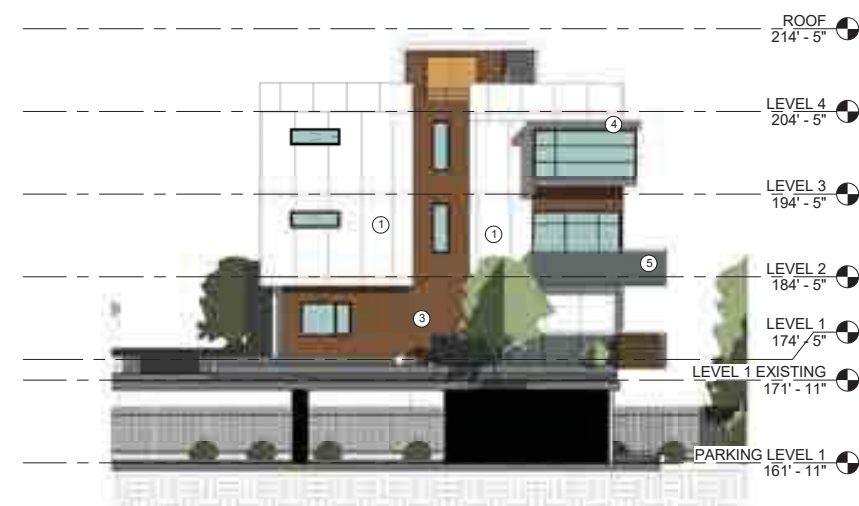
④ Building 4, West Elevation 3/32" = 1'-0"
