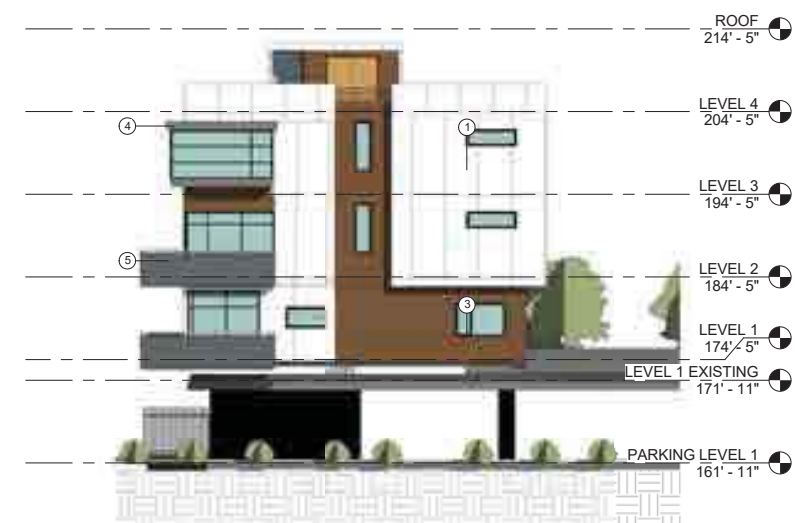
① Building 4, East Elevation 3/32" = 1'-0"
