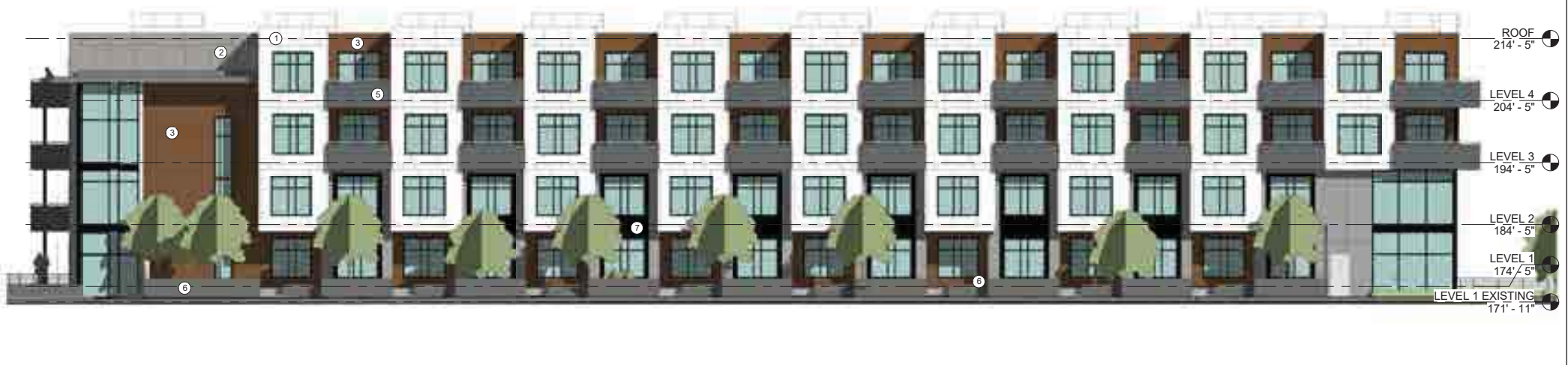
③ Building 1, South Elevation 3/32" = 1'-0"
