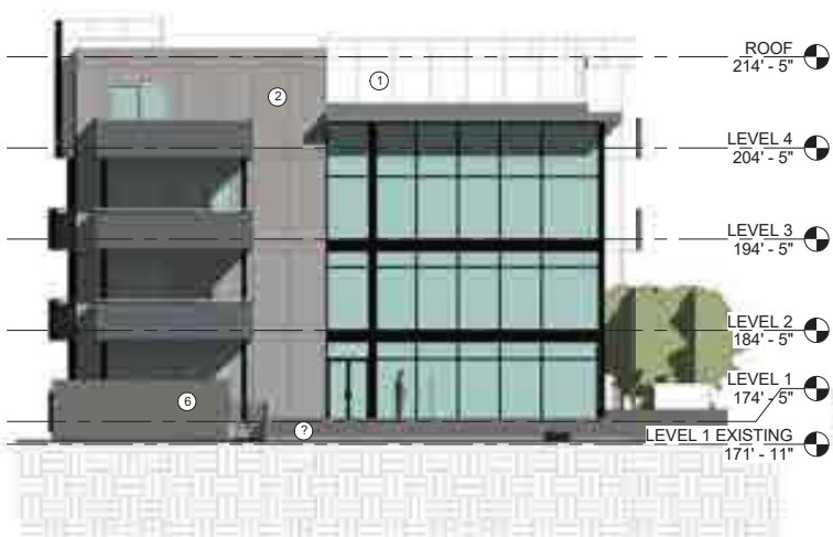
④ Building 1, West Elevation 3/32" = 1'-0"
