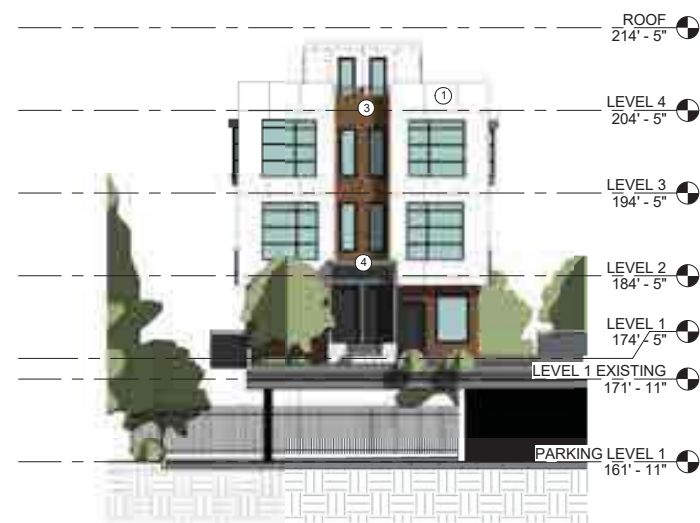
② Building 4, North Elevation 3/32" = 1'-0"
