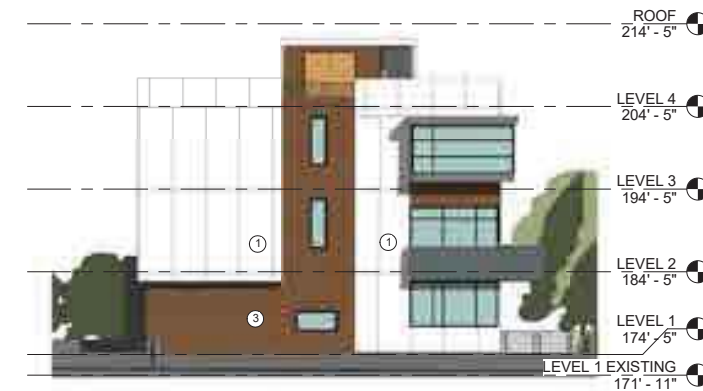
② Building 7, North Elevation 3/32" = 1'-0"
