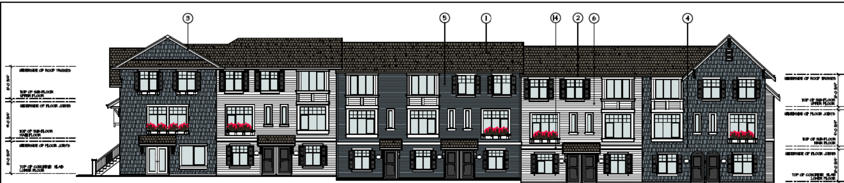
UNIT E * UNIT C1 * UNIT A * UNIT A * UNIT A * UNIT C1 * UNIT C1 * UNIT A * UNIT C1 * UNIT A FRONT ELEVATION SCALE: 1/8" = 1'-0"
