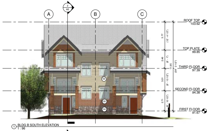
1 BLDG B SOUTH ELEVATION 1:96
