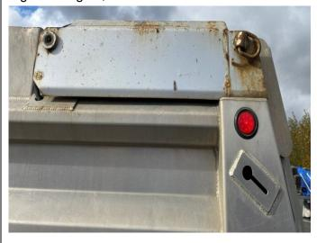
18. Tailgate 44" high, 90 ½" wide, with a lifting bracket in the centre of the tail gate
