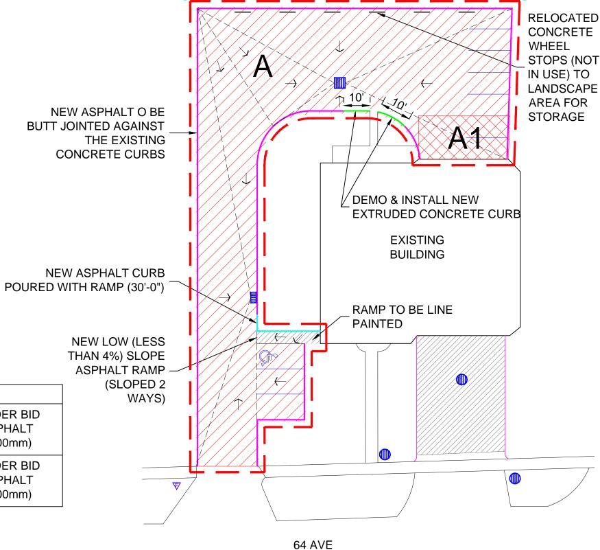
$M^2$  (FT<sup>2</sup>) **TYPE ACTION AREA INCLUDE IN TENDER BID** UPPER/ PRICE (NEW ASPHALT 815 (8,773) Α COURSE#2 THICKNESS = 100mm) **INCLUDE IN TENDER BID UPPER** 55 (592) PRICE (NEW ASPHALT Α1 COURSE #1 THICKNESS = 100mm)
