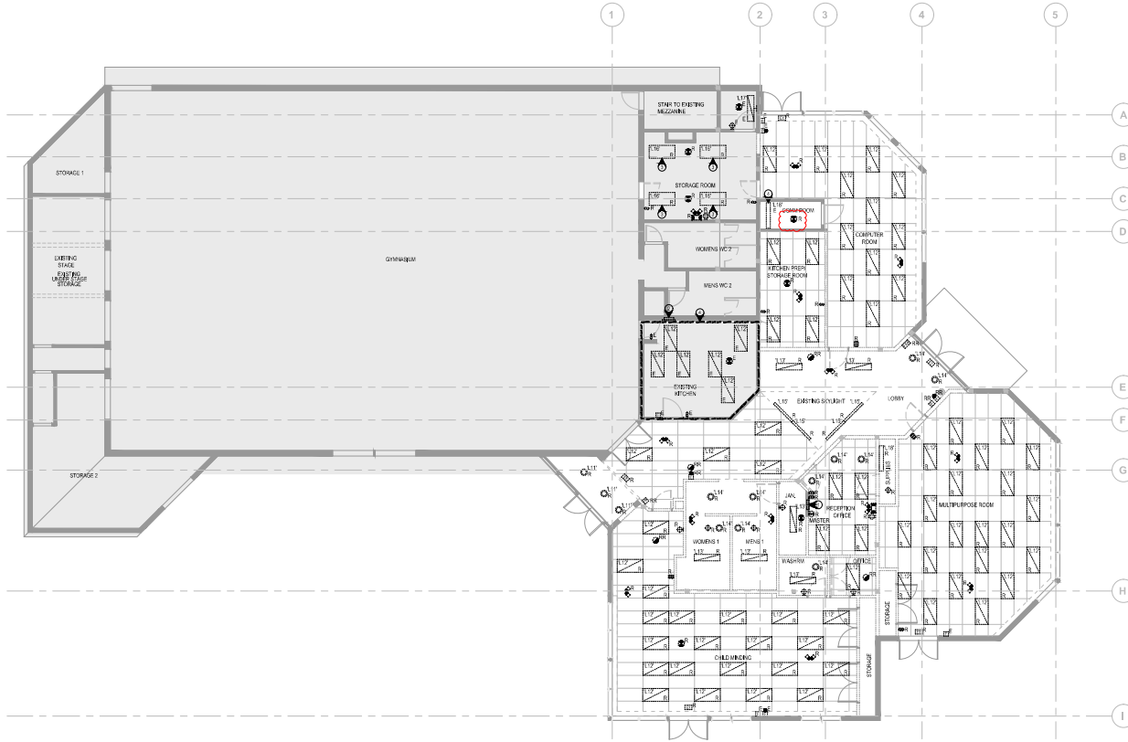
1 E1.0 EXISTING LIGHTING AND LIFE SAFETY LAYOUT 1:100
