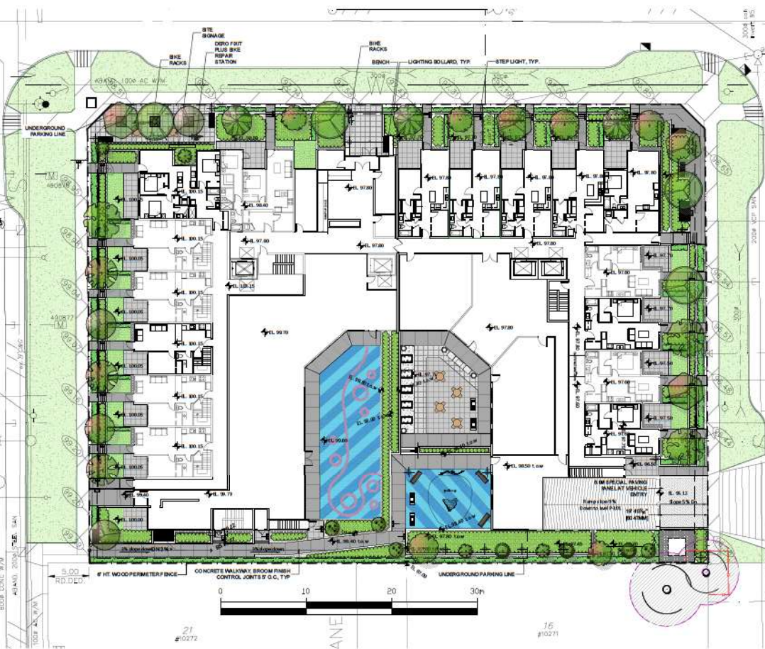
8" FT WOOD PERIMETER FENCE, CONCRETE WALKWAY, BRUSH FINISH, CONTROL JOINTS @ 0.5M, TYP. UNDERGROUND PARKING LINE
