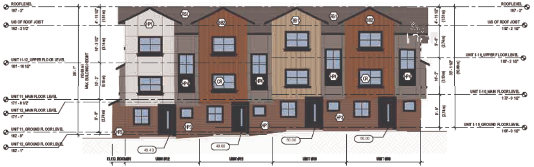
2 BUILDING-03 NORTH ELEVATION SCALE: 1/8"=1'-0"
