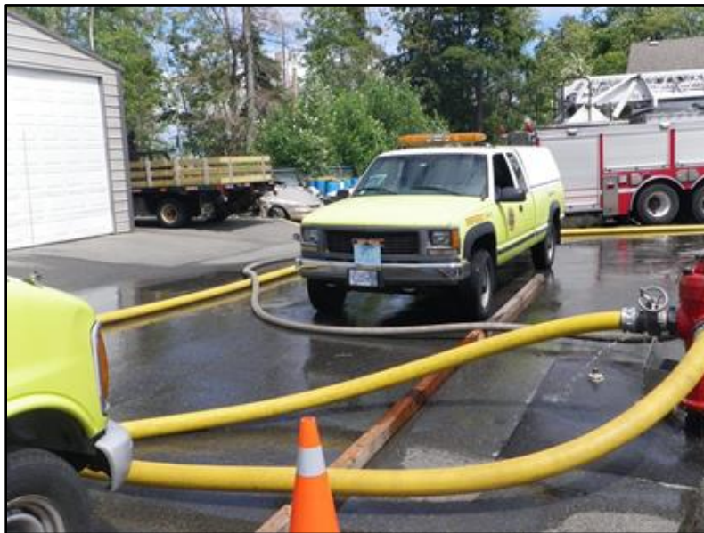
Figure 2: Forward Lay Tactic
