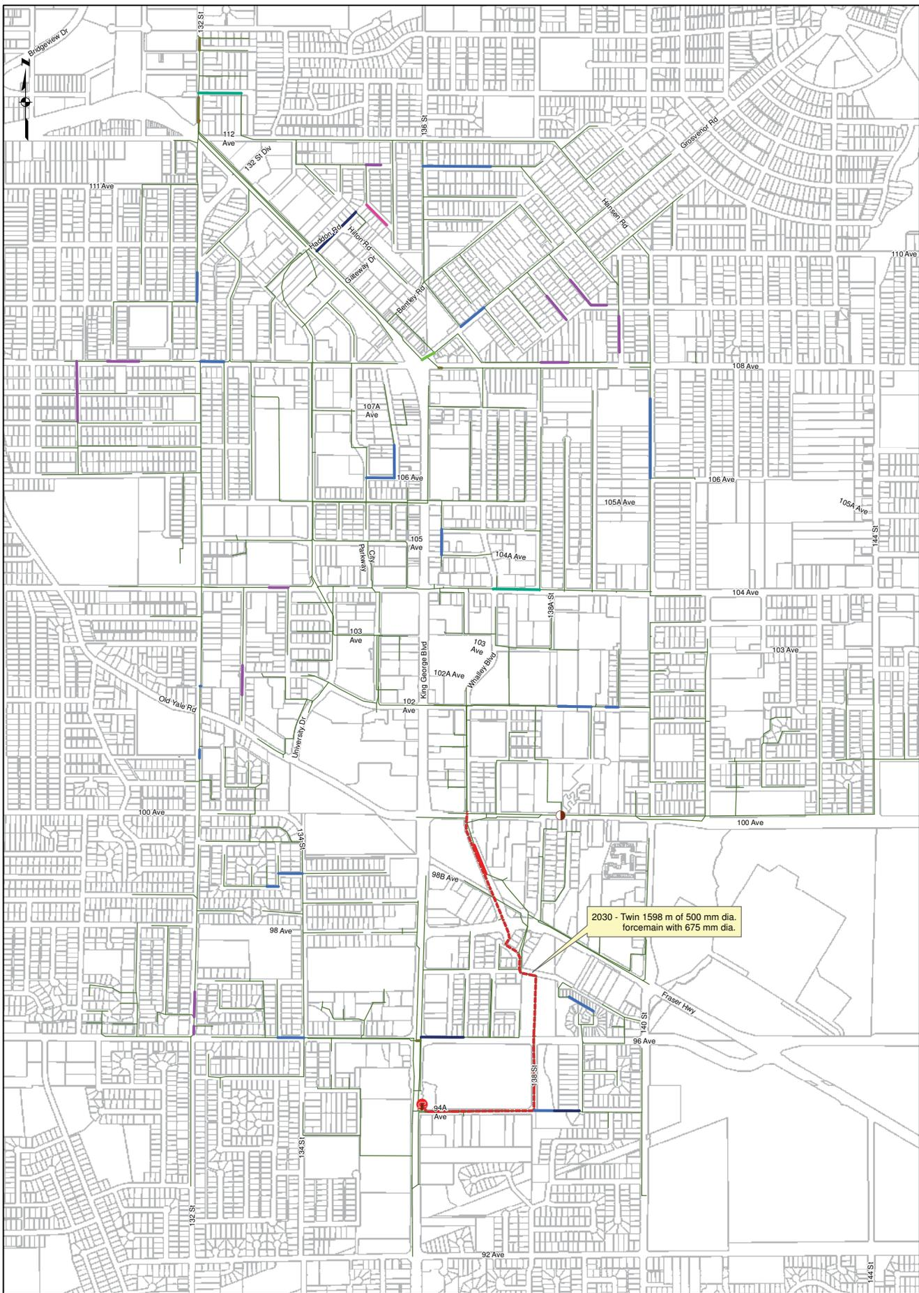
2030 - Twin 1598 m of 500 mm dia. forcemain with 675 mm dia.
