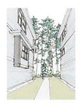
Locate trees no closer than 2 m from a building face, building foundation or
