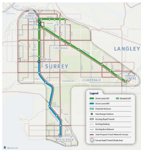
Figure 33: Preferred Rapid Transit Future: Surrey's preferred option within TransLink's option analysis is light rail from City Centre to three town centres: Guildford, Langley City and Newton; and Bus Rapid Transit from Newton to White Rock City Centre. (Map: TransLink / Ministry of Transportation and Infrastructure)
