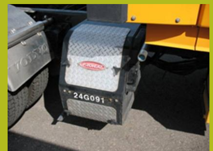
Auxiliary Power Unit on Heavy Duty Truck (Photo: Transport Canada)
