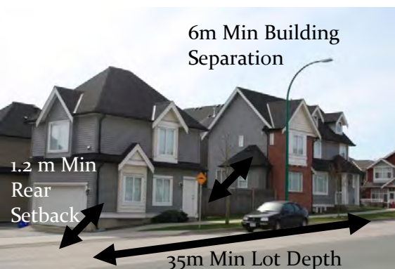
Coach houses provide appropriate Building setbacks and lot depth to accommodate on site yard space.
