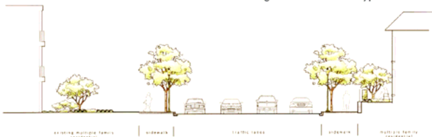
Sketch Section through Martin Drive -- Typical
