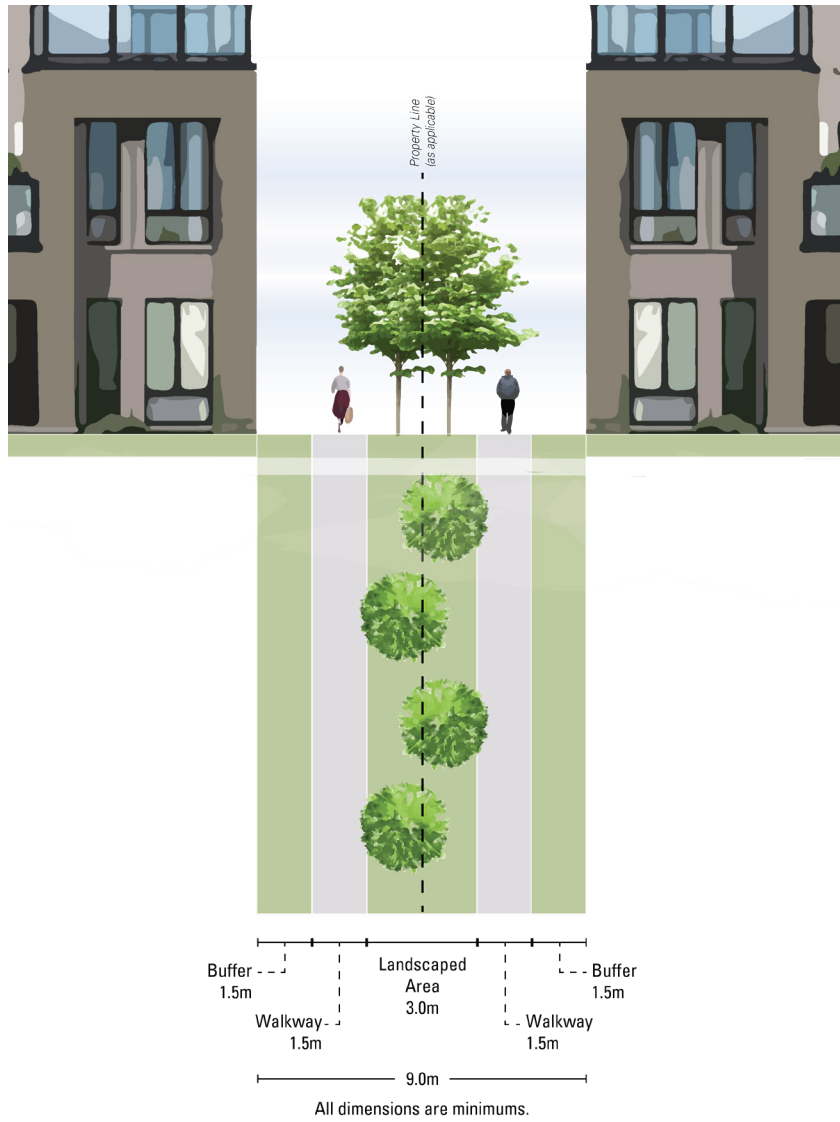
Figure 4.8: Mid-Block Pedestrian Connection Cross-Sections
