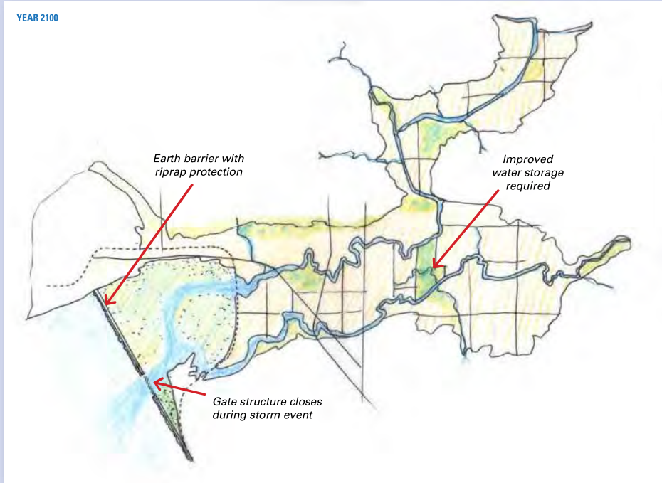
The barrier has minimal impact on reducing waves and relies on a gate structure to minimize the impacts of storm surges. An alternative barrier near shore for Crescent Beach only is shown in Chapter 2.
